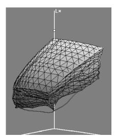
(c) gain in gamut from (a) to (b) Figure 4. Enlarging the gamut of a Color Laser Writer 12/600 PS printer through the black generation
