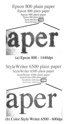
Figure 3. Two sample prints on same type of substrate (plain paper) and with same print mode (best mode) for 2 ink jet printers.
